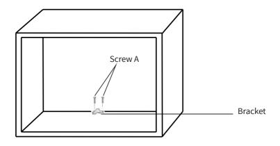
Carefully slide the microwave oven into position making sure that the anti-tilting bracket is locked into the back of the microwave oven. Ensure that the power cord is not taped on kinked.
