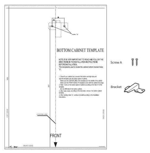
After marking the position of the screws (A) as per the template instructions, remove the template and install the anti-tilting bracket as indicated on the next page.
