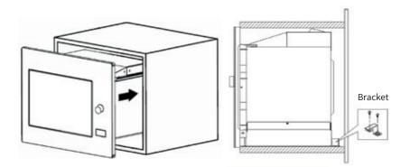
Open the microwave door; install the fixing screw as shown on the image below.
